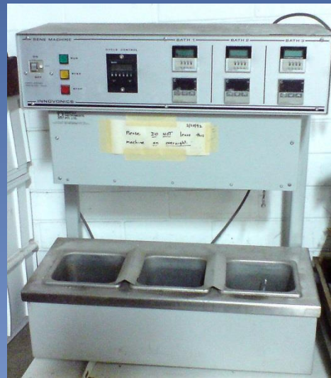
A very early PCR machine Samples moved mechanically
